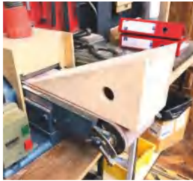
▲ Pic.38 As the drawer wasn't running on rails, I hoped it wouldn't rattle when pulling or pushing. My bets were on oiled timber being smoother to run on
